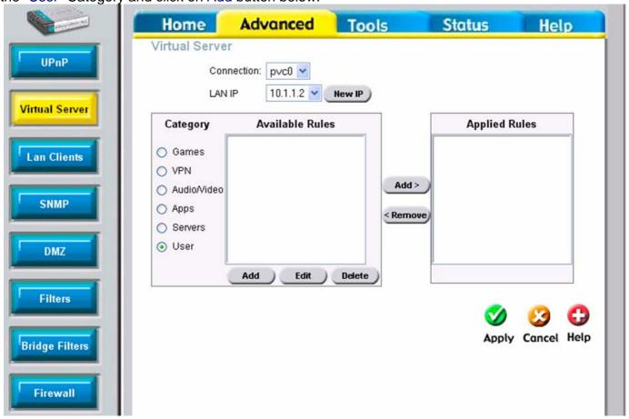
Enter the name for this entry under Rule Name. Then select the necessary protocol (on our case it is TCP). If there is a range of ports to open, specify the starting port under Port Start and the ending port under Port End. If you need to open just one port (like in our example), specify this port in all fields including the Port Map. Click Apply.
