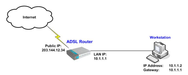
This example shows how to open port 3389 (which is used by Remote Desktop service) in the DSL router running firmware version 2.xx or above. You need to find out what ports your application is using. For example WEB server (HTTP) is using port 80 TCP, PCAnywhere uses ports 5631 TCP and 5632 UDP, etc.
