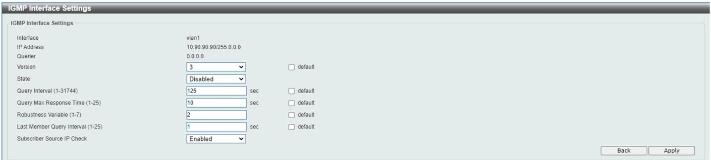
Figure 6-70 IGMP Interface Settings (Edit) Window
