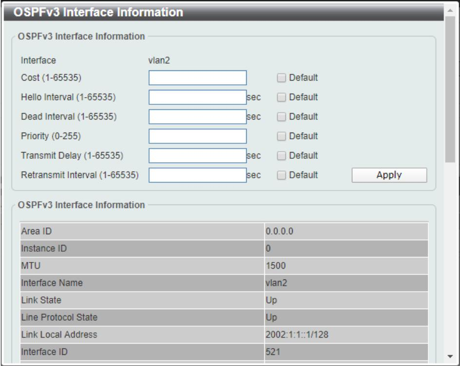
Figure 6-61 OSPFv3 Interface Settings (Interface Name) Window
