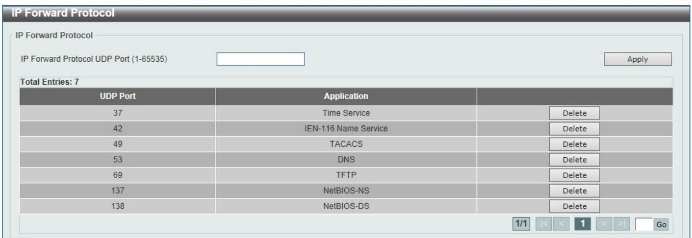
Figure 6-109 IP Forward Protocol Window
