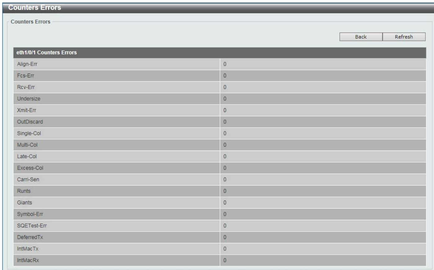
Figure 11-10 Interface Counters (Show Errors) Window
