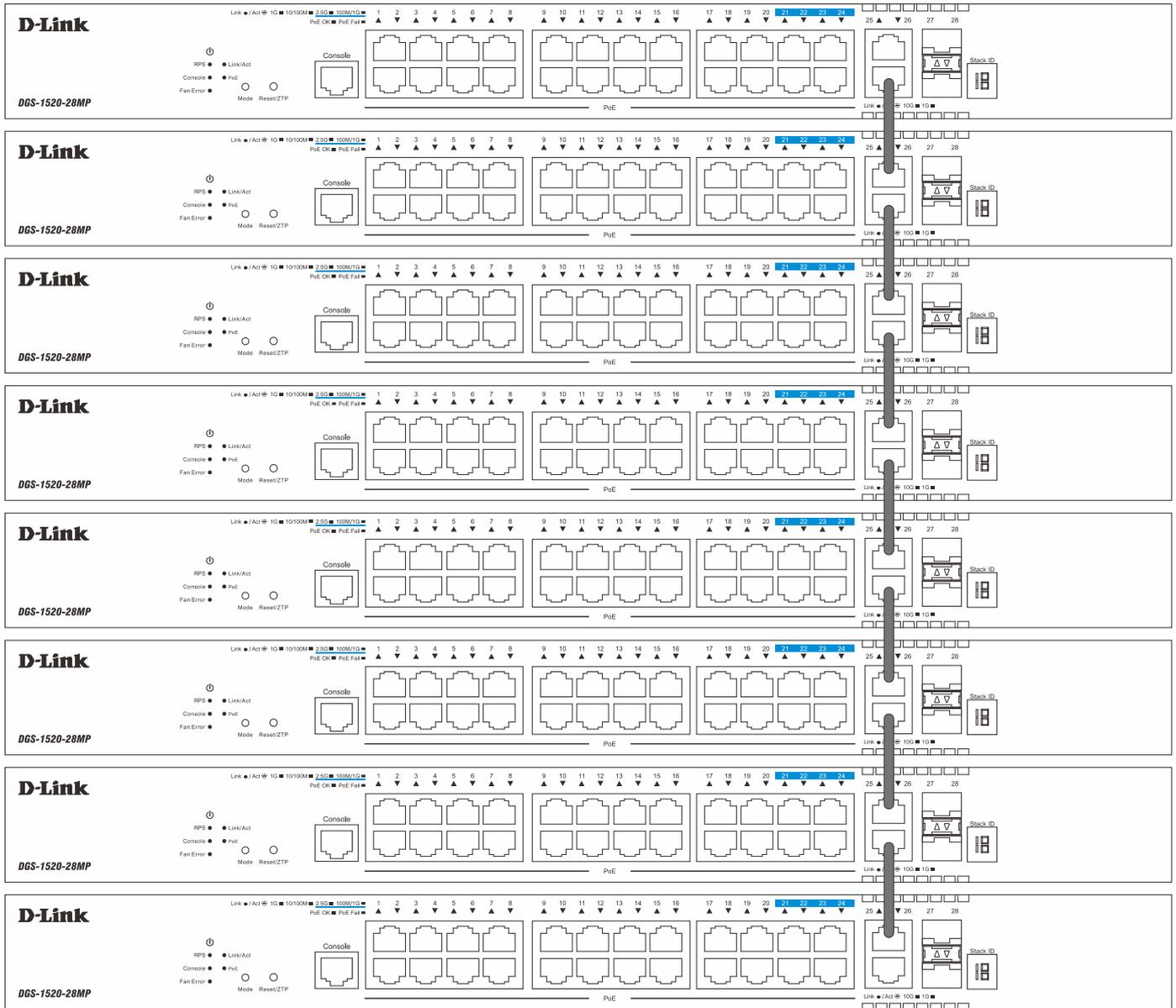
Figure 4-84 Duplex Chain Stacking Topology
