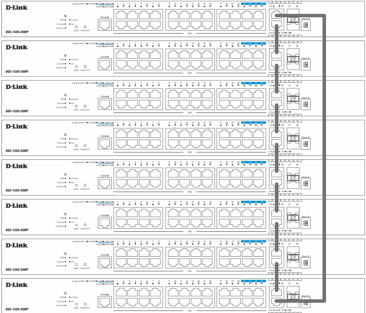
Figure 4-85 Duplex Ring Stacking Topology
