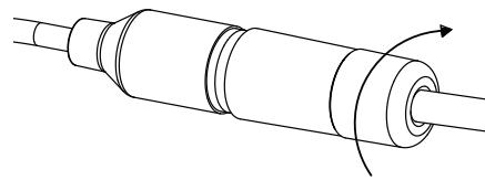
**If you are using PoE to power your camera, use the power connector cap to seal the power connector.**
