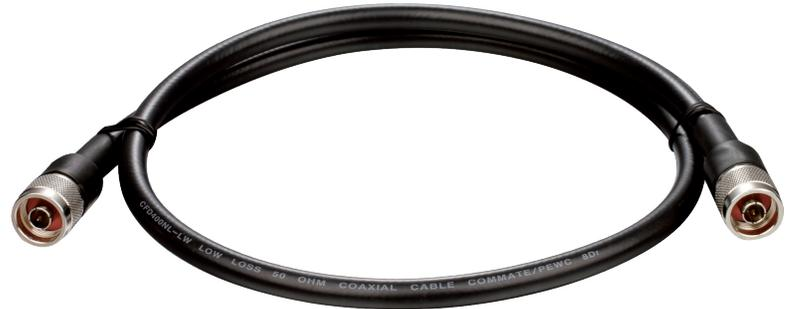
D-Link's ANT70-CB1N and ANT70-CB1RN are one-meter extension cables that connect D-Link outdoor antennas to D-Link outdoor access points. The ANT70-CB1N connects an N plug to an N plug while the ANT70-CB1RN connects a RP-N plug to an N plug. The cables can transmit data with low loss at both 2.4 GHz and 5 GHz. Both cables are certified with the IP67 standard, meaning they are waterproof and dustproof, allowing them to function well in adverse outdoor environments.
